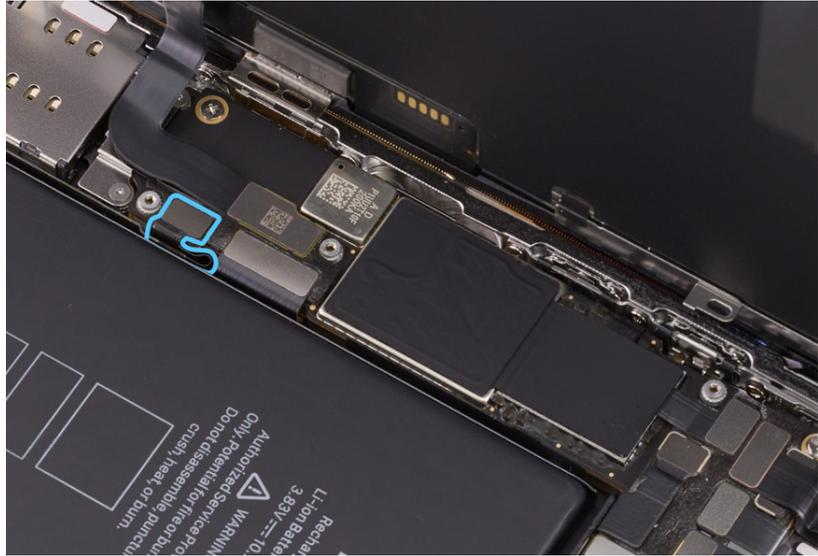
27. Use the black stick to lift the end of the display flex cable off the connector.
