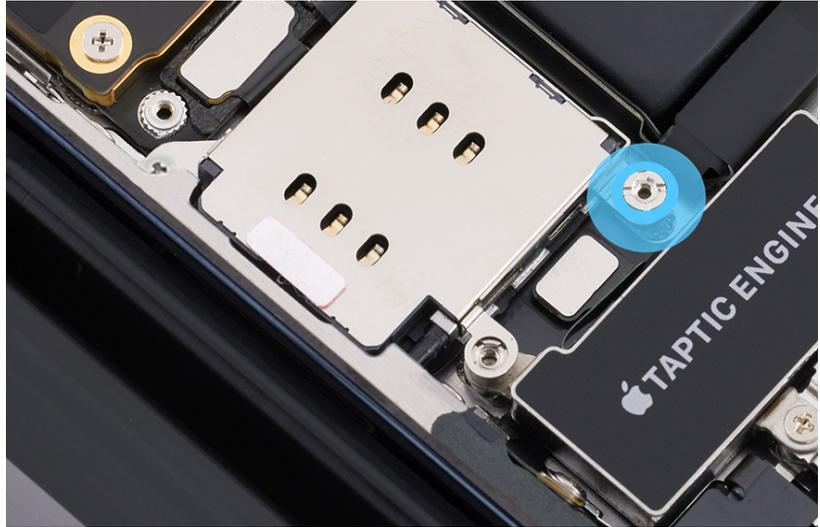
8. Press the end of the SIM reader flex cable to the connector.
