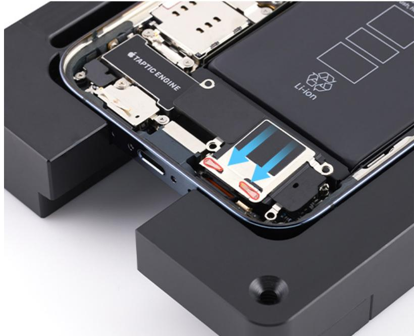
3. Use the green torque driver and JCIS bit to install four new crosshead screws into the speaker.
