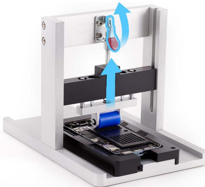
10. Align the right slot on the repair tray with the pin on the battery press.
