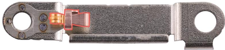
11. Use the black torque driver and Micro stix bit to install four new trilobe screws into the SIM reader and Taptic Engine connector cowlings.
