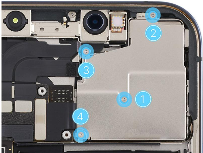
**Reinstall the following part to complete reassembly:**
