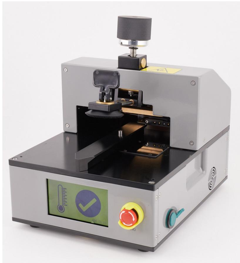
3. Gently insert the iPhone into the heated display pocket with the display faceup and the Lightning connector facing the bottom of the pocket.
