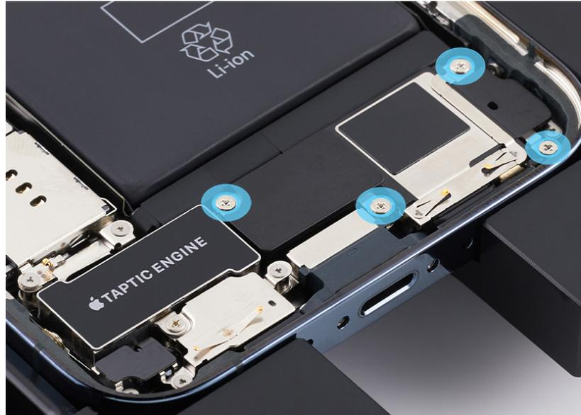
3. Use the black stick to tilt up the speaker. Then remove the speaker from the enclosure.
