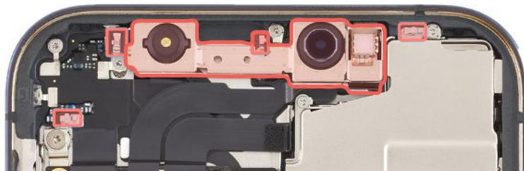
33. Use ethanol wipes or IPA wipes to clean any adhesive residue from the enclosure.
