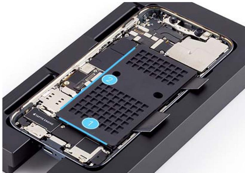
6. Place the repair tray and the enclosure into the battery press. The repair tray has a cutout at the bottom and two slots in the center. Align the left slot on the repair tray with the pin on the battery press.
