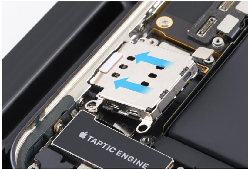
6. Use the black torque driver and Micro stix bit to install one new trilobe screw into the upper left corner of the SIM reader.
