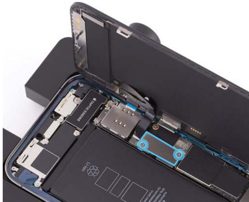
17. The upper cowling has a tab near the second screw hole (2) that fits into a slot near the camera cowling. Use ESD-safe tweezers to fit the tab into the slot. Then lower the cowling over the end of the receiver flex cable.
