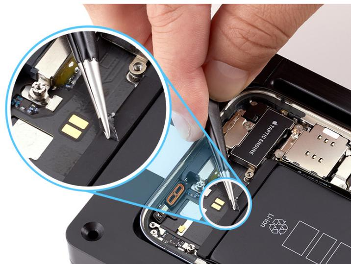
4. Hold down the iPhone. Use ESD-safe tweezers to continue peeling the battery adhesive tab from the battery.
