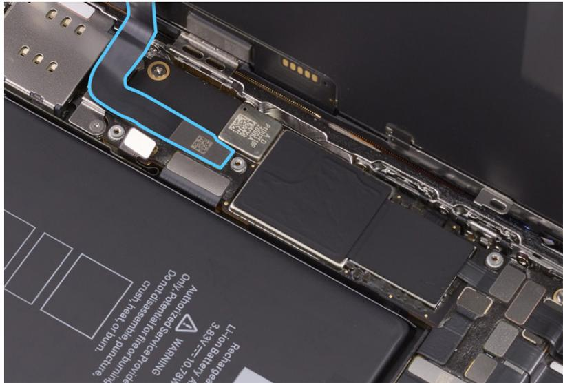
28. Use the black stick to lift the end of the Multi-Touch flex cable off the connector.
