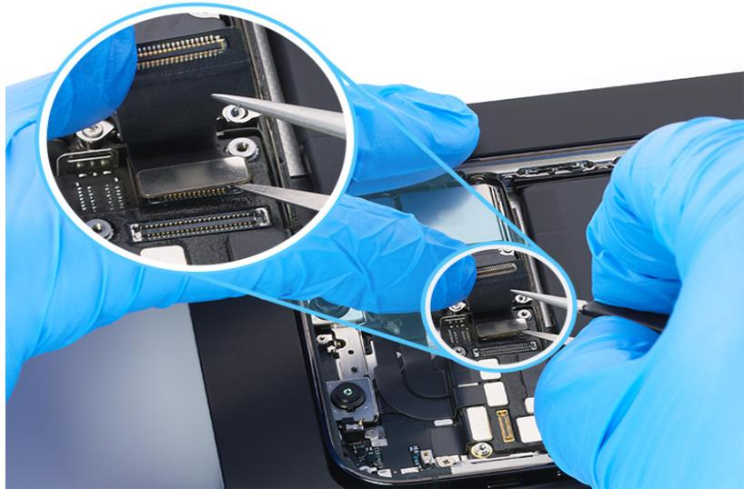
6. Gently hold the flex cables together and lift the cameras out of the enclosure.
