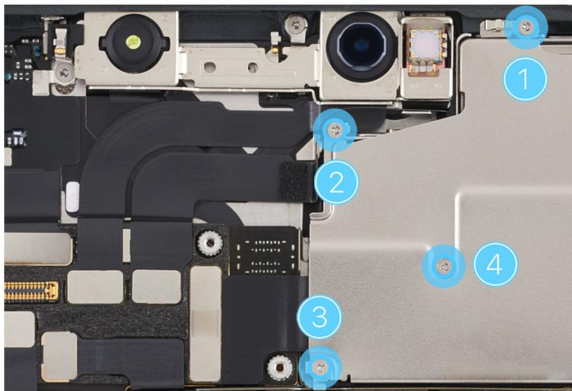
3. Use ESD-safe tweezers to tilt up the left side of the camera cowl as shown. Then slide the camera cowl out of the enclosure. Save the cowl for reassembly.
