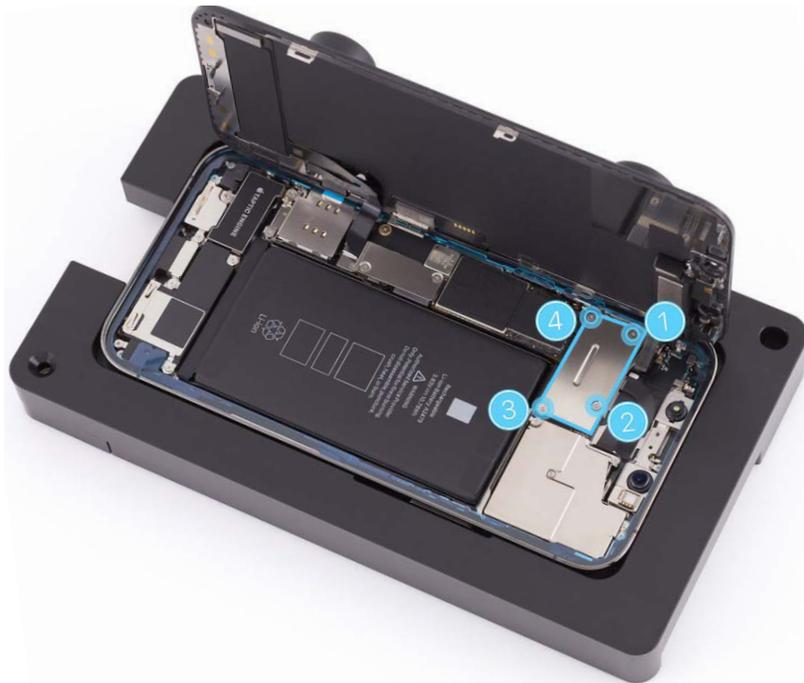
19. Peel the first strip from the middle release liner (1) counterclockwise, starting near the bottom of the right of the enclosure. Peel the second strip (2) clockwise, starting near the bottom right of the enclosure. Peel the third strip (3) counterclockwise, starting near the top left of the enclosure.
