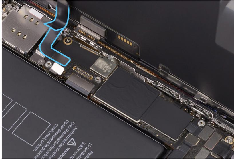
29. Use the black stick to lift the end of the receiver flex cable off the connector.
