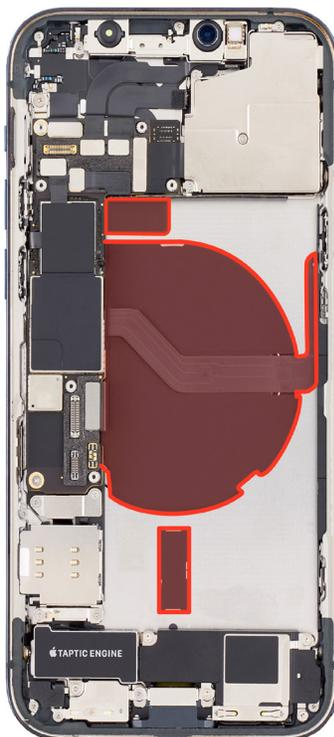
15. Insert the flat end of the black stick into one of the insertion points as shown. Ensure that the black stick is inserted into a point where the battery strip has been fully removed. Don't insert the black stick into a point where the battery tab or strip is broken.
