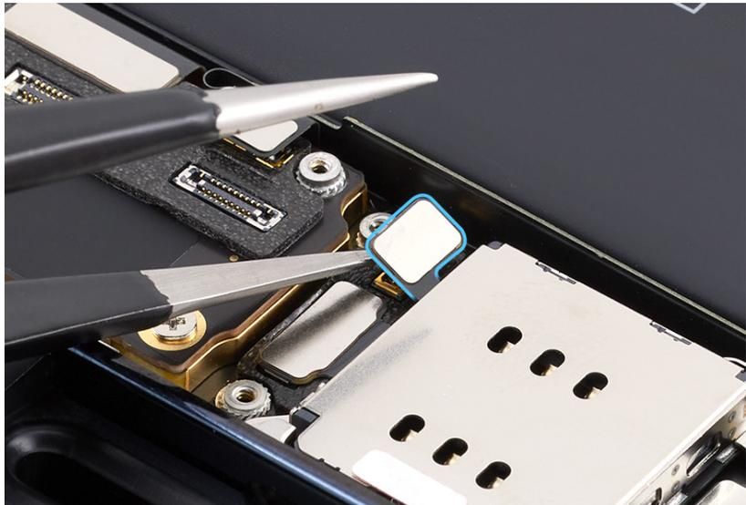
9. Use a torque driver and the Micro stix bit to remove the trilobe screw from the upper left corner of the SIM reader. Set aside the screw.
