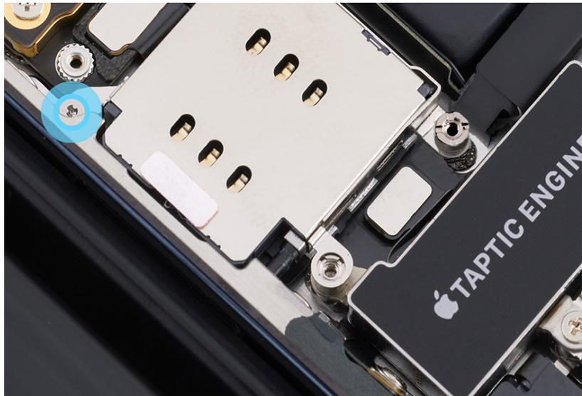
7. Use the gray torque driver and super screw bit to install one new super screw into the lower right corner of the SIM reader.
