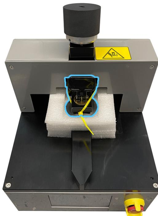
3. Turn the top knob on the fixture counterclockwise to raise the suction cup. Remove the packing Styrofoam.
