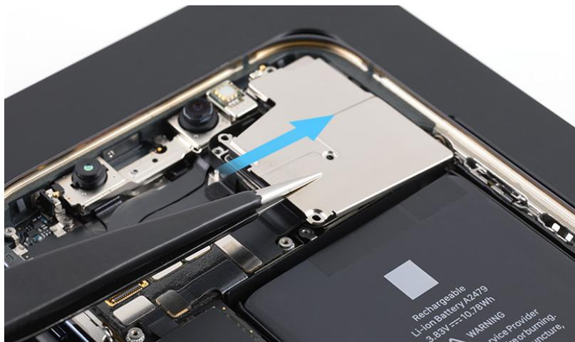
8. Use the black torque driver and Micro stix bit to install four new trilobe screws into the camera cowling in the order shown.
