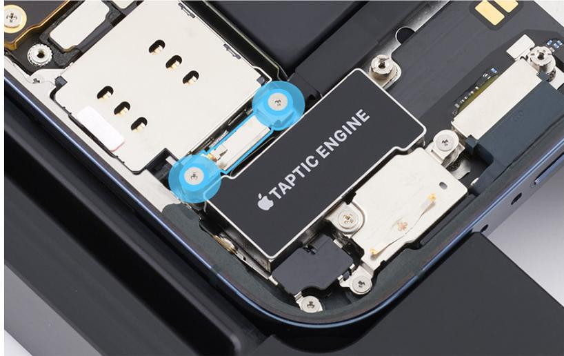
7. Use ESD-safe tweezers to remove the Taptic Engine connector cowling. Save the cowling for reassembly.
